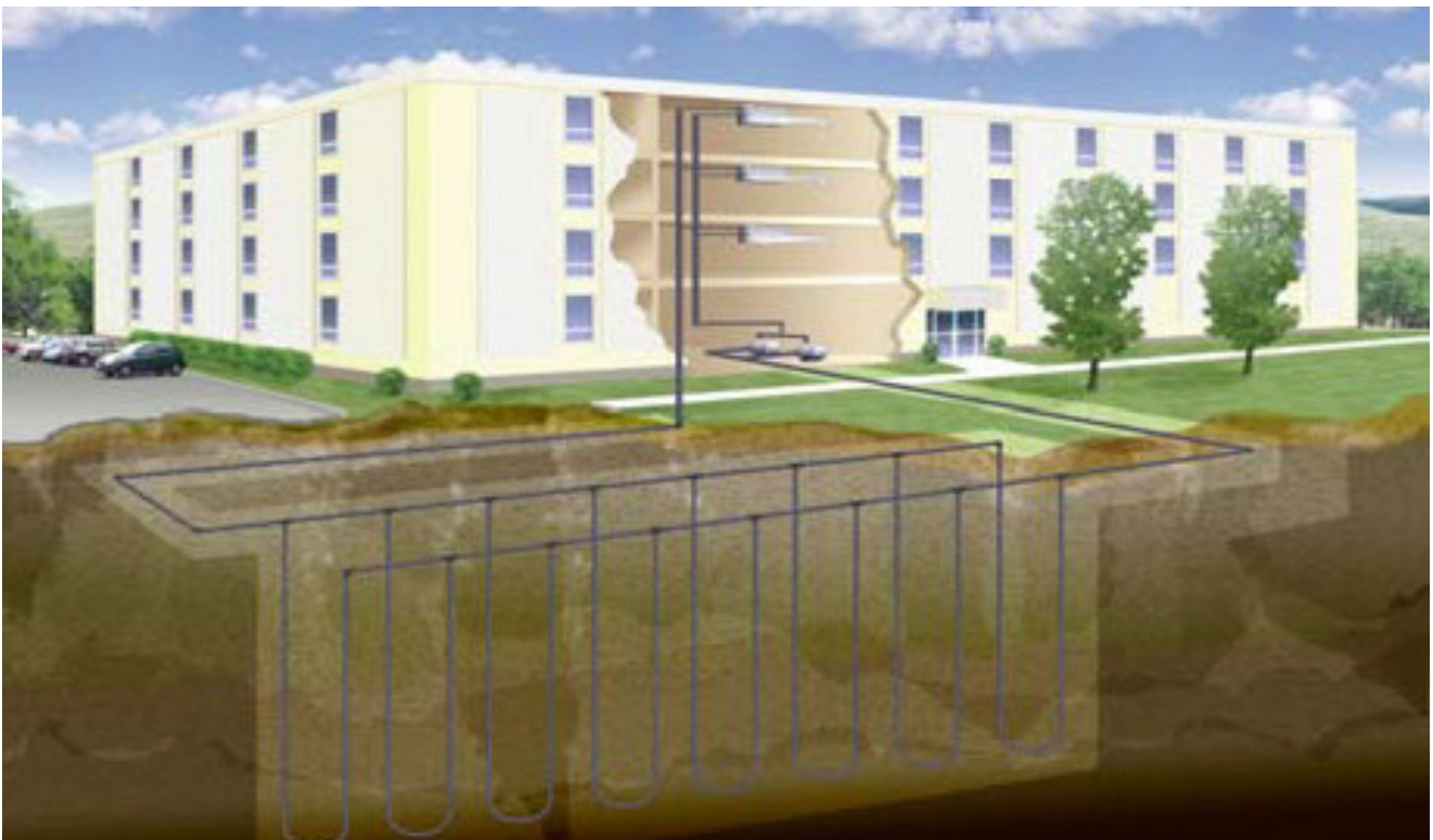
DIAGRAM OF A TYPICAL VERTICAL, CLOSED-LOOP SYSTEM
