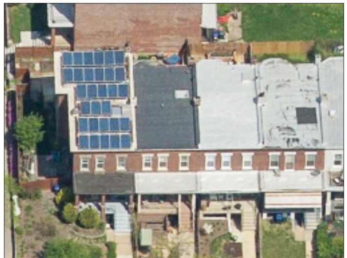
VISIBILITY OF SOLAR PANELS ON THIS CORNER ROWHOUSE WOULD BE DIMINISHED IF THEY WERE SETBACK FROM THE FRONT OF THE ROOF EDGE.
