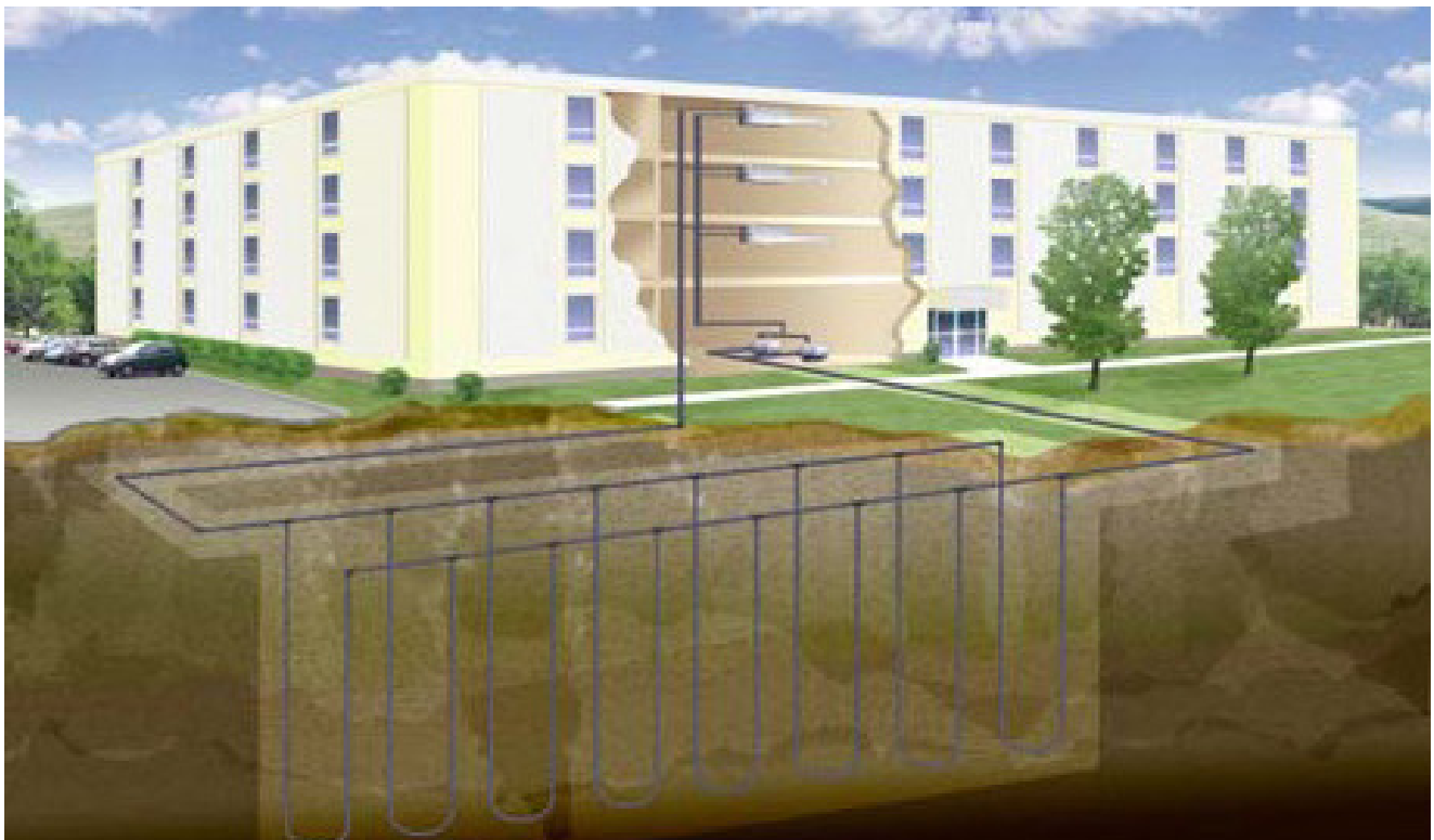
DIAGRAM OF A TYPICAL VERTICAL, CLOSED-LOOP SYSTEM
