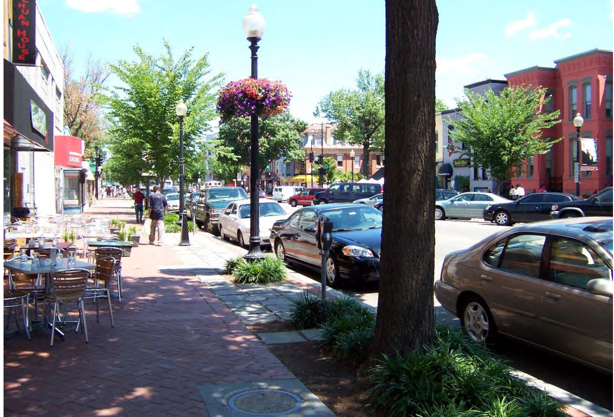
The tree box area in commercial areas with high pedestrian traffic may be paved with a permeable pattern of brick, flagstone, or concrete pavers.
