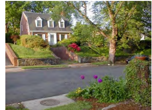
Plantings in the tree box area should have shallow roots and grow less than 18 inches.
