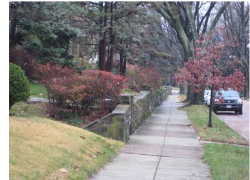
The 6 foot sidewalk width in residential areas is in part intended to make paving secondary to landscaping.
