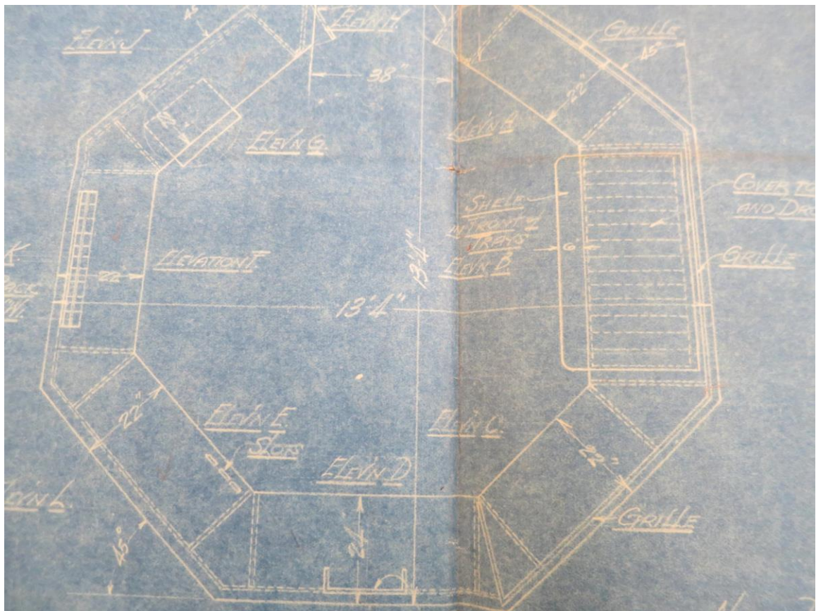
Photo 22. Southeast Branch Library, Washington, D.C. Blueprint for the construction of the octagonal special charging desk on the main level. See 1968 photo of interior *. DC Library Archives, 1922.
