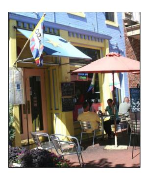
Shed-style awnings and canopies are generally the most appropriate form for a flat-topped opening. Awnings and canopies should only be attached to a building in a manner that does not cause permanent damage, generally not through masonry. Awnings and canopies should have a minimum clearance height of 8'.
