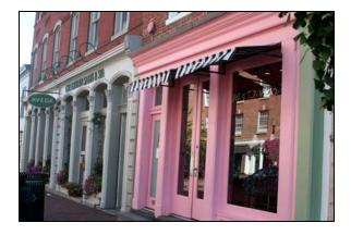
The size, shape, and proportions of original storefront windows should be maintained, and new windows should match the originals as closely as possible. Unless they are replacing originals, replacement windows should be fixed (not operable); should not be divided up into smaller panes; and should have a thin window frame profile.
