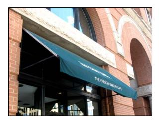
Awnings should relate to and fit within the masonry or frame openings of a window or door and should not cover over character-defining features of a historic building.
