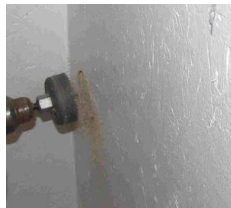
Figure 2-14. Drilling second calibration hole
