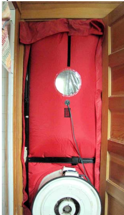
Figure 2-6. Blower Door Installed in Bathroom Doorway
