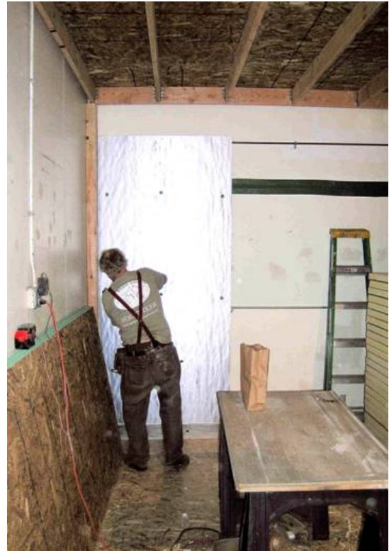
The photo on the left shows three walls of the chamber completed with the test cell inside. The outer chamber, likewise well insulated and sealed, is cooled while the test cell is heated to test U values.
