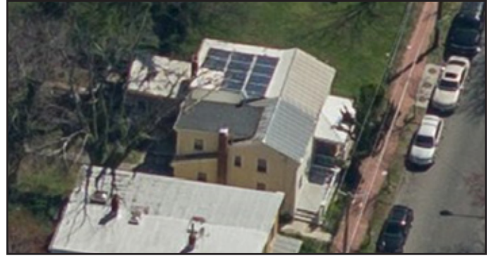
Solar panels on the rear roof slope of this semi-detached house are installed flush to the roof and setback from edges minimizing visibility from the street.
