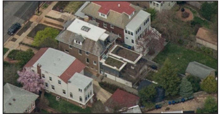
This example took advantage of a rear addition, reducing visibility and avoiding removal of original building materials.
