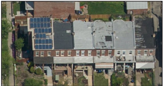
Visibility of solar panels on this corner rowhouse would be significantly improved if they were setback from roof edges.
