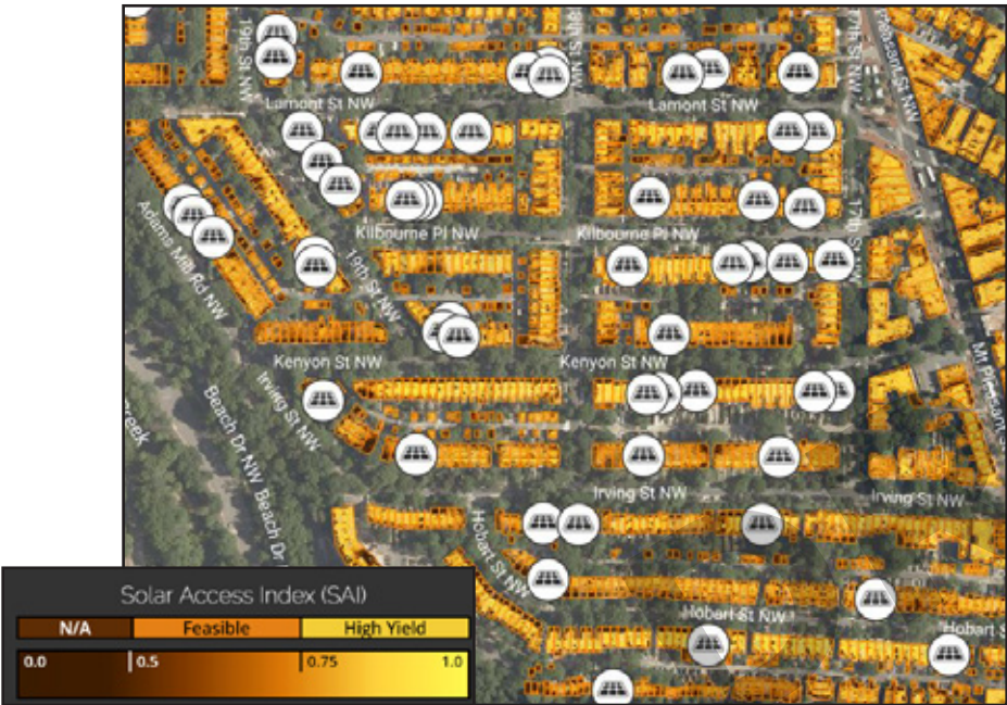
Mapdwell Solar System(left) is an interactive online rooftop solar mapping tool that allows users to determine their rooftop solar potential as well as where solar has been installed elsewhere in their community.
