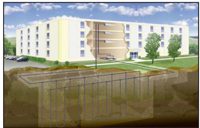
Diagram of a typical vertical, closed-loop system.
