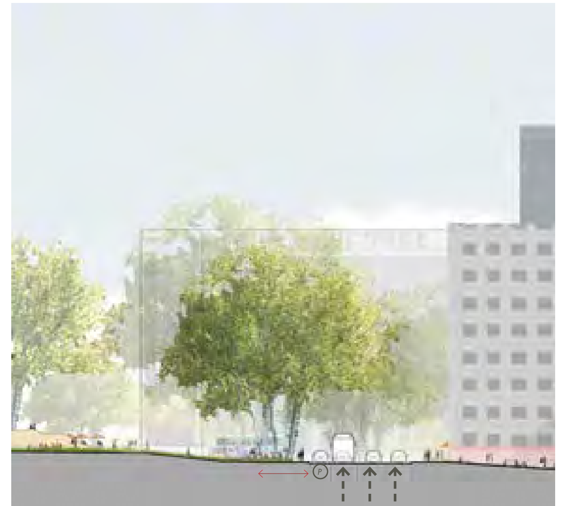
Potential section through K Street NW south of Mount Vernon Square. One-way circulation, reduced roadway width and midblock crosswalks make pedestrian crossings easier. An expanded sidewalk allows additional room for pedestrians, bike movements.
