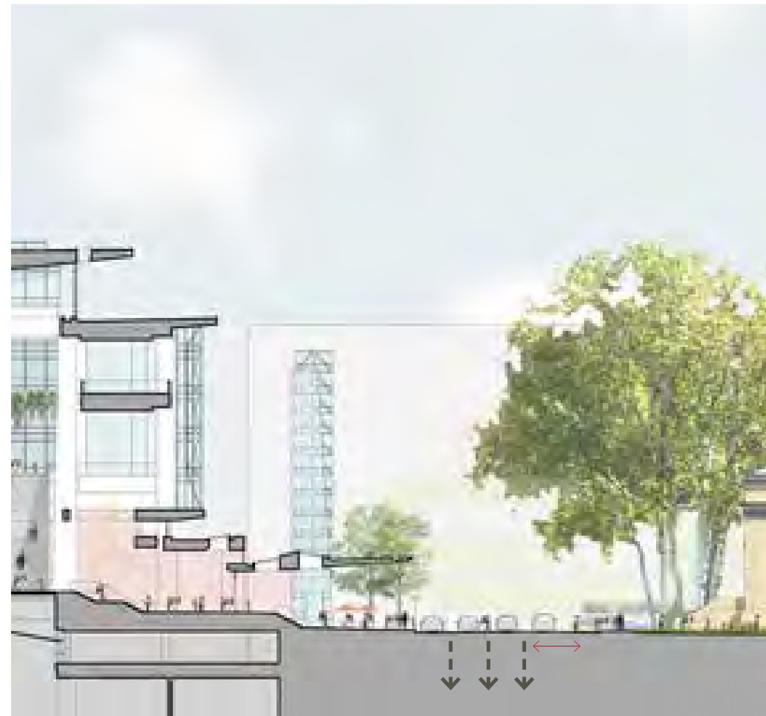
Potential section through Mount Vernon Place NW. One-way circulation, reduced roadway width and a midblock crosswalk make pedestrian crossings easier. An expanded sidewalk allows additional room for pedestrians on the square.
