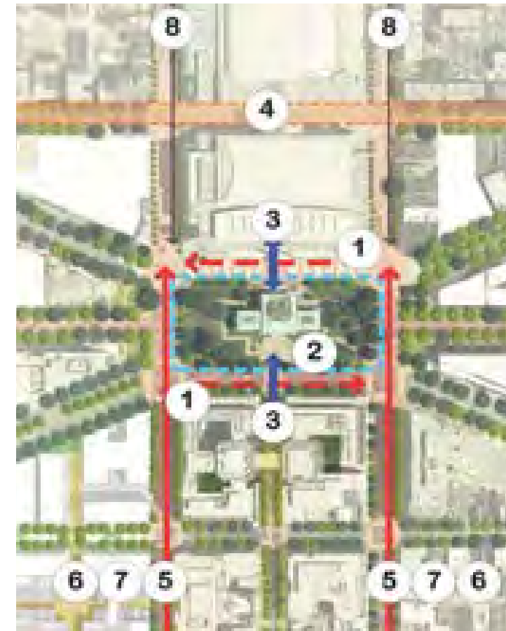
A PARTIAL ONE-WAY LOOP FOR MOUNT VERNON SQUARE, 7TH AND 9TH STREETS NW
