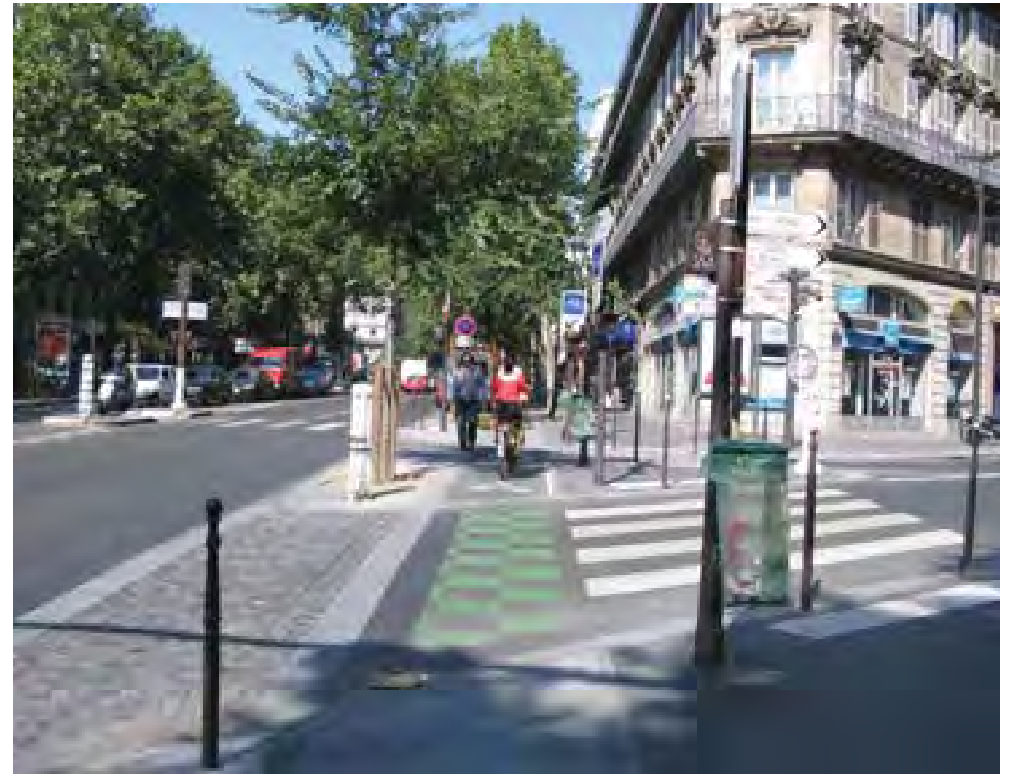
Above: crosswalk in Paris. Well marked crosswalks make circulation for pedestrians and bicyclists safer; their high visibility ensures that motorists can see them. Signage clearly directs bicyclists to a specific zone so as to minimize conflicts and safety features such as bollards enhance pedestrian comfort levels.
