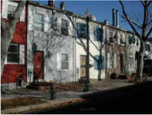
Projections are limited to uncovered steps on narrow streets.
