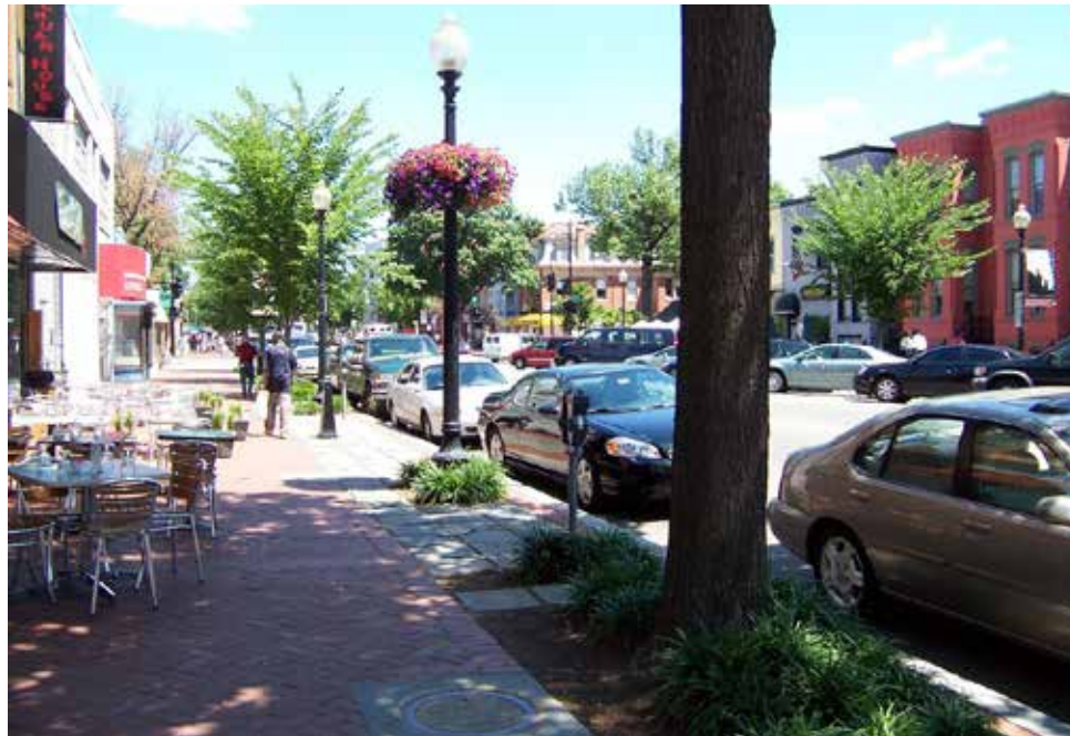
The tree box area in commercial areas with high pedestrian traffic may be paved with a permeable pattern of brick, flagstone, or concrete pavers.
