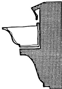
External gutters are attached to eaves of sloping roofs.
