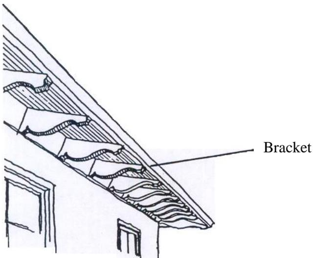
An eave visually terminates the top of a wall.
