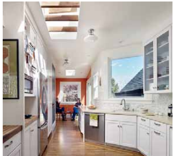
Skylights can deliver natural sunlight into the interior of a rowhouse, reducing the cost of interior lighting and improving summertime ventilation.
