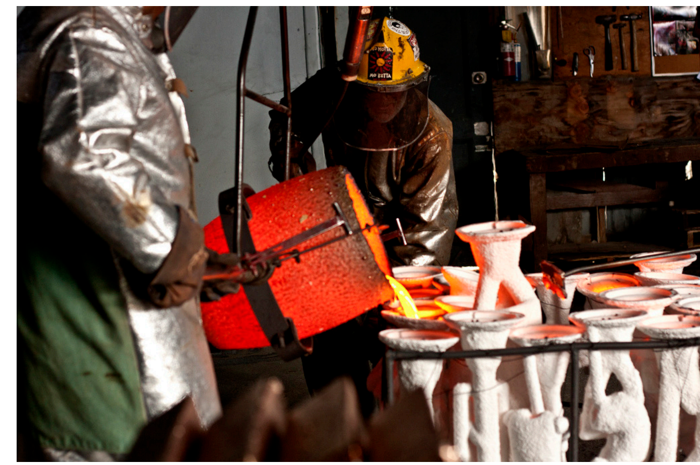
Workers at Artwork Foundry on Heinz Fill Casts with Molten Bronze. (Photo: John Osborn)
