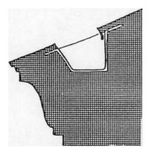
Internal gutters are located within eaves of sloping roofs.
